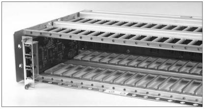
**INSERT ETHERNET MODULES IN SLOTS 1-4 (Red)**
